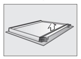
■ Remove the glass fibre seal. To do so pull the ends out of the fixings at the side.
